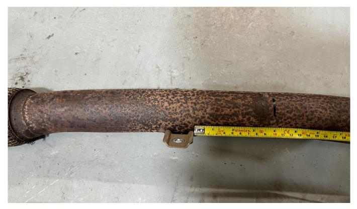
Cut the original exhaust system 100mm after the front mounting bracket as per the photo above.
